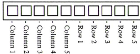
Figure 4-1 Keypad Connector
