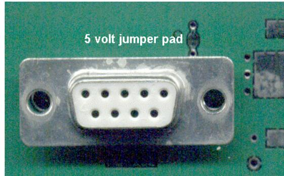
To use pin 9 as the power source, the user must solder the 5 volt jumper pad beside the DB9 connector. If you have any further questions or concerns don't hesitate to contact Matrix Orbital at support@matrix-orbital.com.
