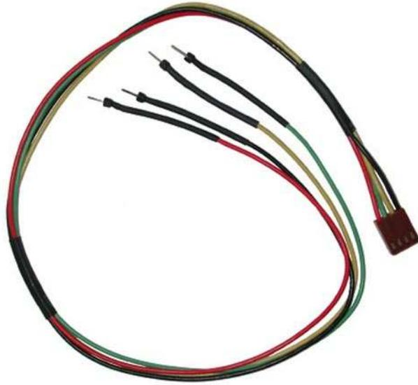
Figure 5: Breadboard Cable
