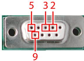
Figure 10: DB9 Pinout
