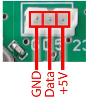
Figure 16: 1-Wire Pinout
