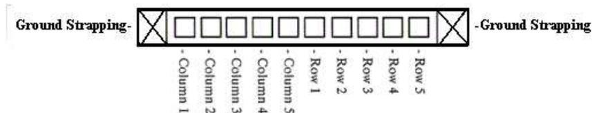
Figure 21: Keypad Connector
