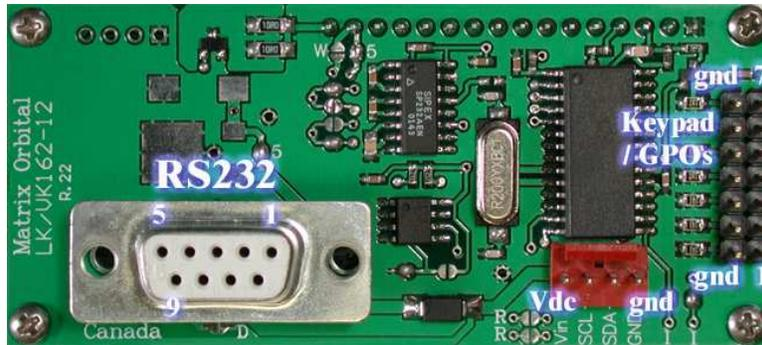
Figure 4: Electrical Connections
