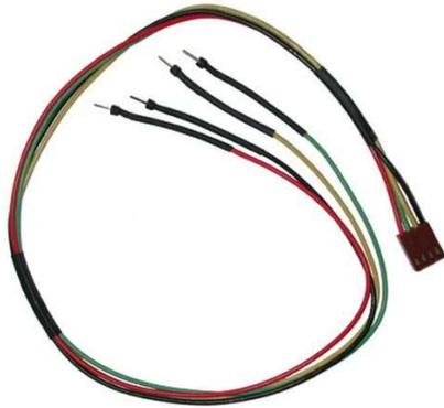
Figure 3: Breadboard Cable
