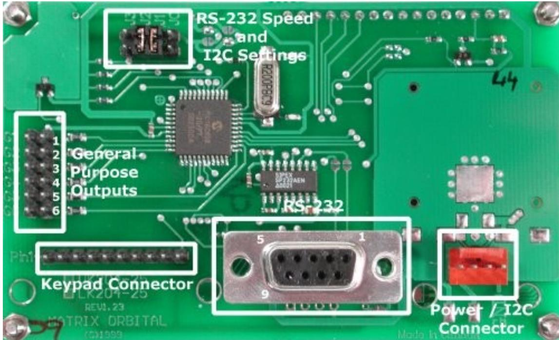
Figure 2-2 Electrical Connections
