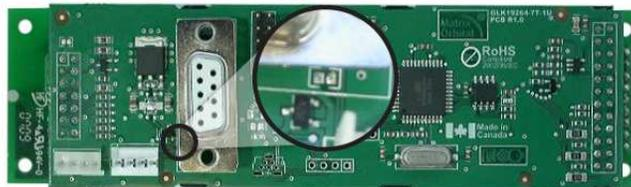
Figure 14: Power Through DB-9 Jumper
