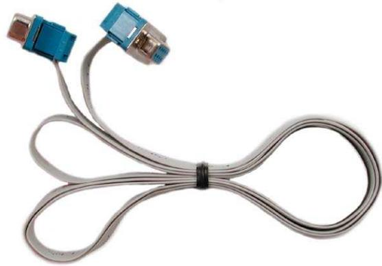
Figure 8: Serial Cable
