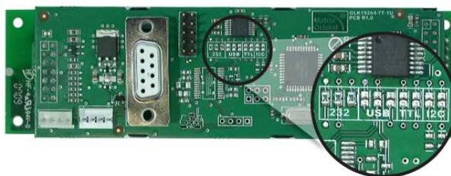
Figure 17: Protocol-Select-Jumpers for GLK19264-7T-1U Non-USB
